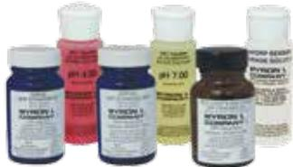
The ULTRAPEN™ PTBT3 requires Myron L® Company 80mV Quinhydrone, 260mV Quinhydrone, or 470mV MLC Light's ORP Standard Solutions for wet calibration and Sensor Storage Solution for proper storage.
