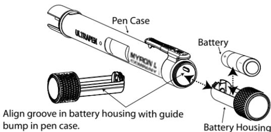
1. In a CLEAN DRY environment unscrew the PT3 battery cap in a counter-clockwise motion.
