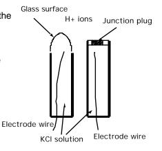
limits the lifetime of a pH junction from depletion of solution inside the reference junction or from contamination. The junction is damaged by drying out because insoluble crystals may form in a layer, obstructing contact with test solutions. See Cleaning Sensor, pg. 10.
