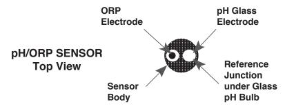
Leaving high pH (alkaline) solutions in contact with the pH sensor for long periods of time is harmful and will cause damage. Rinsing such liquids from the pH/ORP sensor well and refilling it with Myron L Storage Solution, a saturated KCl solution, pH 4 buffer, or a saturated solution of table salt and tap water, will extend the useful life.
