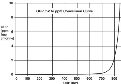
\*Given water is sanitized by only chlorine at a pH of 5-9 and a temperature of 20-30°C
