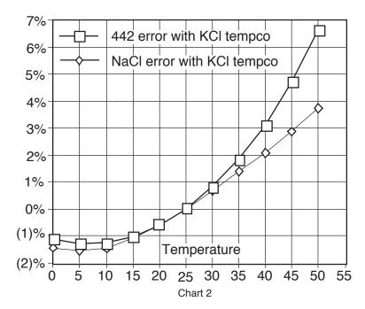
Users wanting to measure natural water based solutions to 1% would have to alter the internal compensation to the more suitable preloaded "442" values or stay close to 25°C. Users who have standardized to KCl-based compensation may want to stick with it, regardless of increasing error as you get further from 25°C. The Ultrameter II will provide the repeatability and convertibility of data necessary for relative values for process control.
