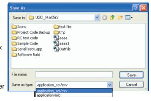
format. If the .csv format is chosen, then the data will be saved as the scientific data format without truncating any data. CSV (comma separated values) data format can be read by many spreadsheet programs, e.g., Microsoft Excel™. In Mac OSX this function is the same as "Save".
