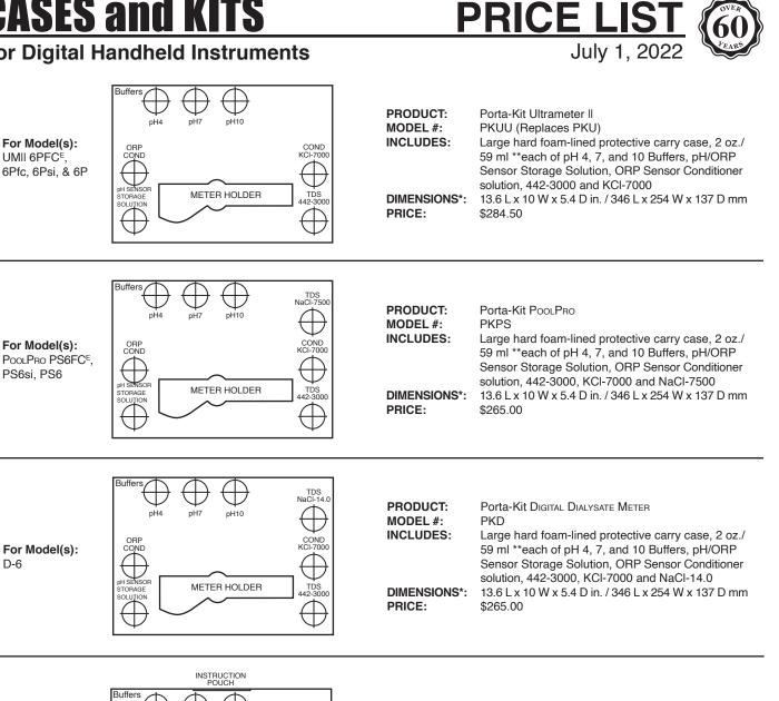
PRODUCT: Litho-Kit Ultrameter II MODEL #: ULK pH4 pH10 Syringe Large hard foam-lined protective carry case, 2 oz./ INCLUDES: 59 ml \*\*each of pH 4, 7, and 10 Buffers, pH/ORP For Model(s): CONE KCI-700 Thermomete UMII 6PFCE Sensor Storage Solution, ORP Sensor Conditioner solution, 442-3000 and KCI-7000, graduated 35CC 6Pfc, 6Psi, & 6P syringe and thermometer METER HOLDER **DIMENSIONS\*:** 13.6 L x 10 W x 5.4 D in. / 346 L x 254 W x 137 D mm PRICE: \$354.00
