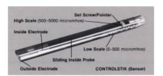
Bring Controlstik (sensor) electrodes together by sliding the inside probe completely forward. Use a screwdriver
