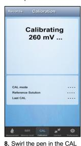
solution while the PTBT4's LED is flashing rapidly.
