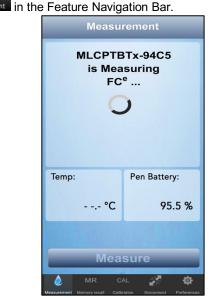
5. Swirl the pen in the sample while the PTBT4 is measuring. The PTBT4's LED will flash rapidly.
