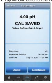
**14.** When the 2nd CAL point is finished, place the PTBT4 sensor in the remaining pH Buffer, then tap CONTINUE.
