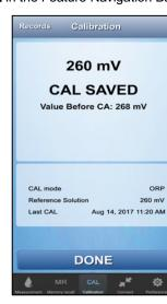
When the Calibration is done the App displays the values and saves a CAL record.
