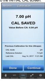
13 When the 1st CAL Point is finished, place the PTBT4 sensor in either 4.0 or 10.0 pH Buffer, then tap CONTINUE.
