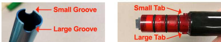
2. While maintaining alignment, gently apply pressure to insert the sensor into the ULTRAPEN. You may need to apply a slight twisting motion to start each O-ring, ensuring all 3 O-rings on sensor slide evenly into ULTRAPEN. **CAUTION:** A damaged O-ring will allow solution to leak into the instrument. Press sensor **STRAIGHT** into the ULTRAPEN until it is securely in place.
