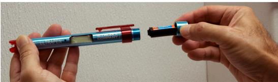
5. Grasp the sensor body and gently pull the sensor out of the ULTRAPEN.
