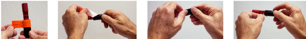
2. If there are salt crystals around the cap of the sensor, using caution not to allow the connector side of the sensor to get wet or contaminated, carefully rinse sensor with clean water, shake off excess water, and dry the outside of the sensor body. Remove the connector cap from the connector end of the sensor and inspect to ensure 3 O-rings are on the sensor body.
