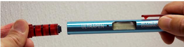
6. Carefully clean off any residual salt or liquid around the opening of the ULTRAPEN's sensor compartment using a towel. **CAUTION:** Do NOT contaminate the inside of the ULTRAPEN.
