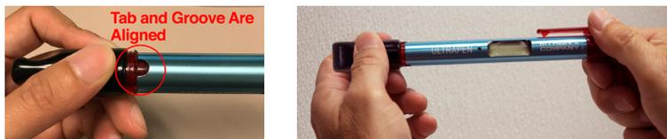
3. Replace the battery tray by aligning the guide bump inside the enclosure with the alignment groove in the battery tray, then sliding the tray into the case until it is fully seated. The groove in the tray corresponds to a guide bump inside the enclosure that guides the tray back into the correct position. Screw the battery cap back on.
