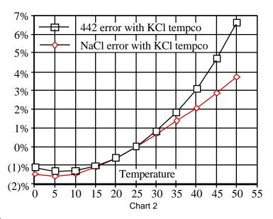
Users wanting to measure natural water based solutions to 1% would have to alter the internal compensation to the more suitable preloaded "442" values or stay close to 25°C. Some who have standardized to KCl based compensation may want to stick with it, regardless of increasing error as you get further from 25°C. The AR1 will provide the repeatability and convertibility of data needed for relative values for process control.
