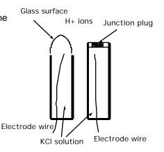
limits the lifetime of a pH junction from depletion of solution inside the reference junction or from contamination. The junction is damaged by drying out because insoluble crystals may form in a layer, obstructing contact with test solutions. See pH, pg. 15.
