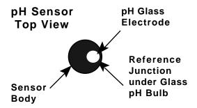
Samples containing chlorine, sulfur, or ammonia can "poison" any pH electrode. If it is necessary to measure the pH of any such sample, thoroughly rinse the pH sensor well with clean water immediately after taking the measurement. Any sample element which will reduce (add an electron to) silver, such as cyanide, will attack the reference electrode.
