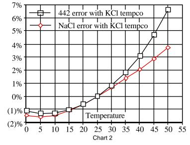
Users wanting to measure natural water based solutions to 1% would have to alter the internal compensation to the more suitable preloaded "442" values or stay close to 25°C. Some who have standardized to KCI based compensation may want to stick with it, regardless of increasing error as you get further from 25°C. The ARH1 will provide the repeatability and convertibility of data needed for relative values for process control.
